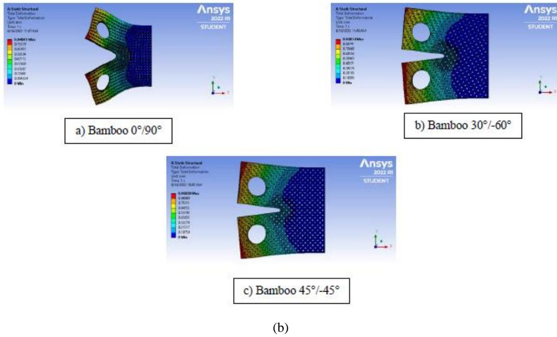
**Fig. 3.1 - Total deformation simulation results (a) Bamboo fiber; (b) Kenaf fiber**
