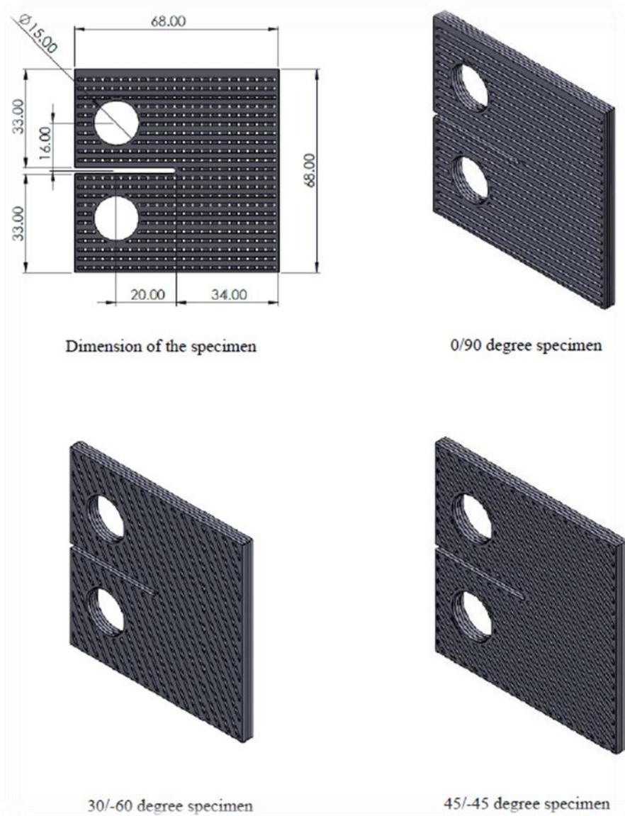
**Fig. 2.1 - Geometry of the woven orientation specimens**
