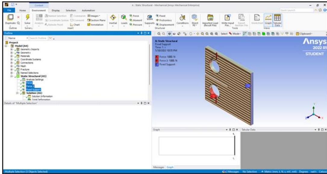
Fig. 2.2 - Boundary condition of all the specimens
