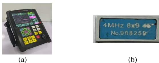
Fig. 1 - The main equipment used for ultrasonic testing (a) rigor RFD 60 was the equipment used for UTFD in this study; (b) probe 4MHz with 45°
