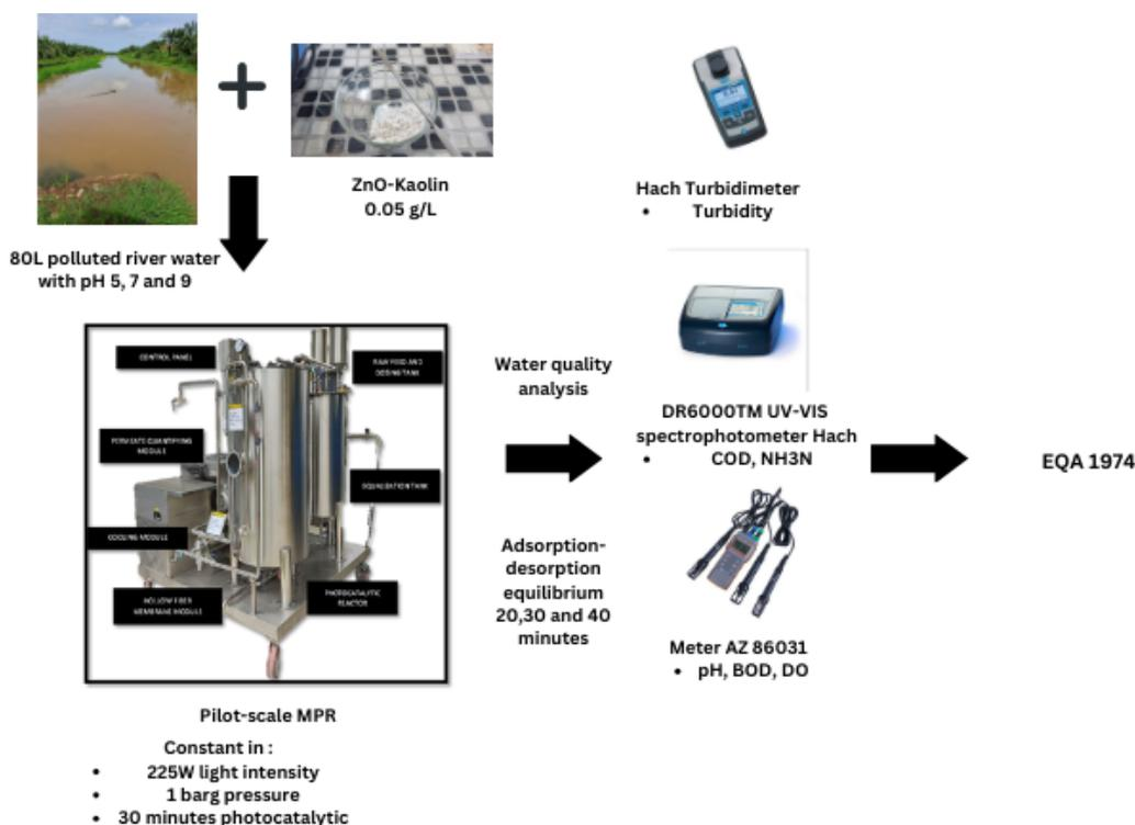
Fig. 1 Apparatus in analysing the quality of river water
