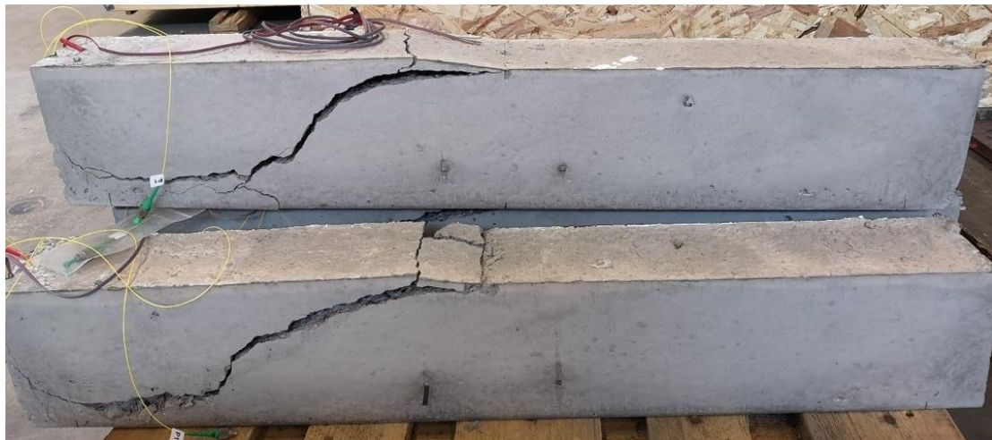
Fig. 1 - Concrete beam specimens after testing. The shear failure mechanism occurs [29]
