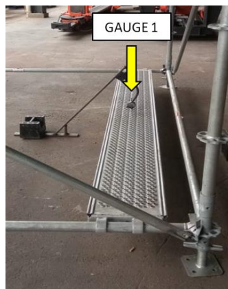
Fig. 4 - Dial gauge installation for individual platform
