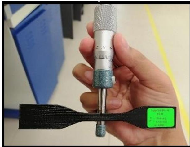
Fig. 5 - Measuring reduced section width of specimen test
