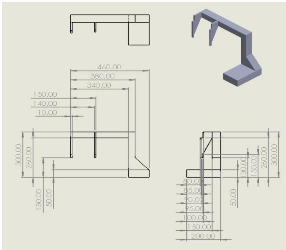
**Fig. 6 - Seatbelt release mechanism design using SolidWorks**
