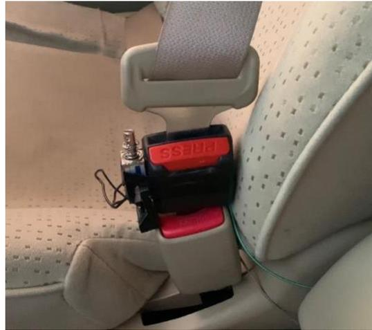
**Fig. 14 - Solenoid hold down the release mechanism to unlock the seatbelt**
