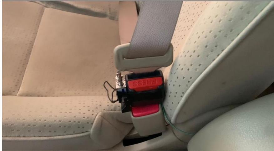
**Fig. 11 - The seatbelt auto release mechanism is installed to buckle**
