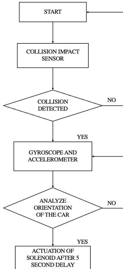
Fig. 4 - Algorithm used in the proposed system
