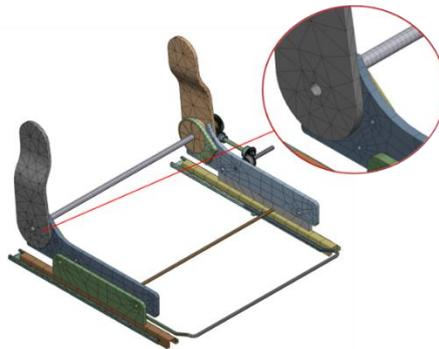
**Fig. 4 - Mesh generated of seat models**
