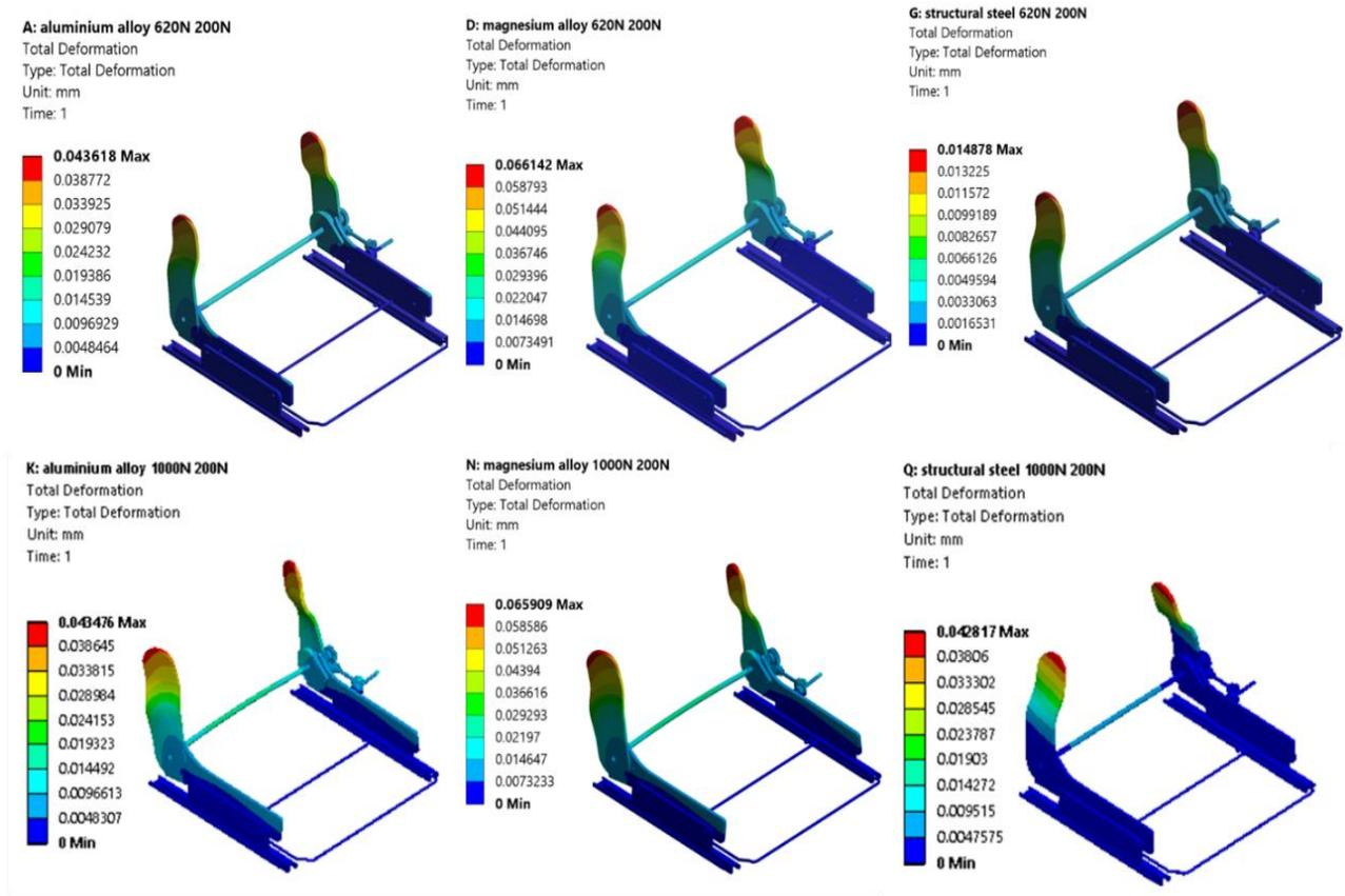
Fig. 7 - Total deformation result at structural analysis
