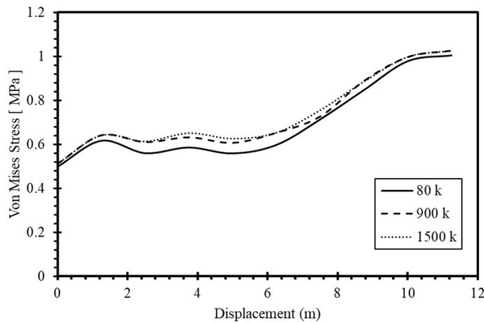
**Fig. 6 - Grid Independence Test result with three different elements number**
