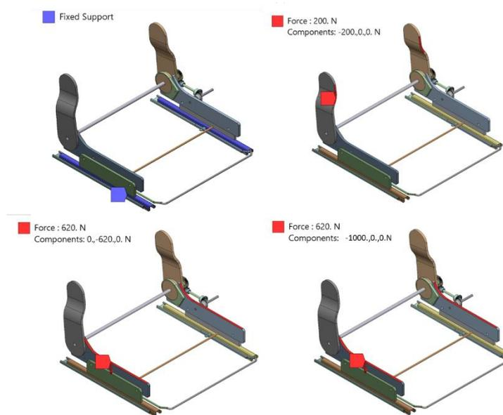
**Fig. 5 - Constraint conditions for force applied**
