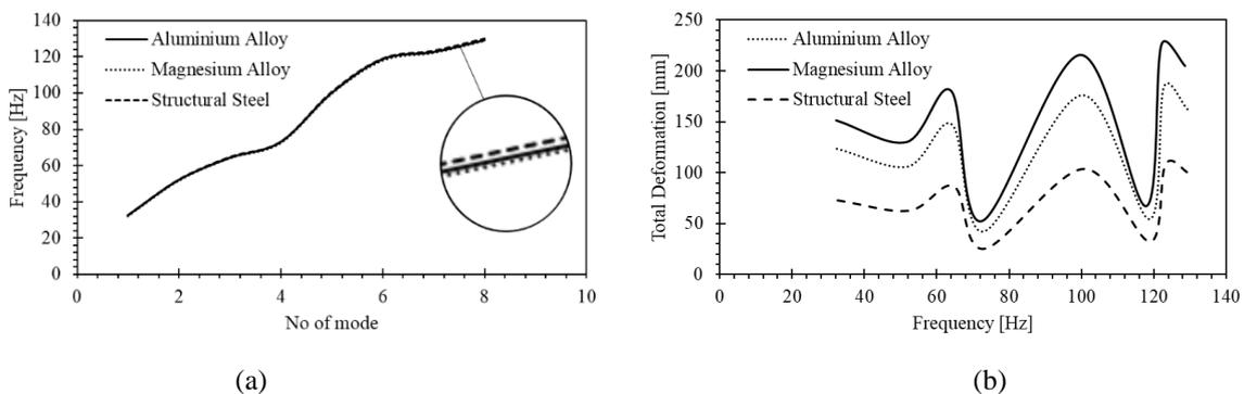
Fig. 9 - (a) Value of frequency from no of mode; (b) total deformation graph for different material
