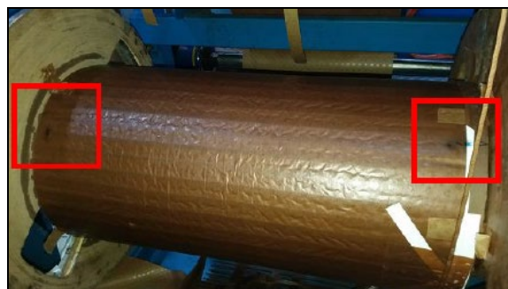
Fig. 2.7 - Points of punctures of a coil between HV and LV coil barrier sheet
