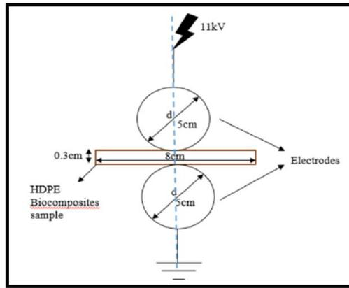
Fig. 1 - Geometry of electrode configuration
