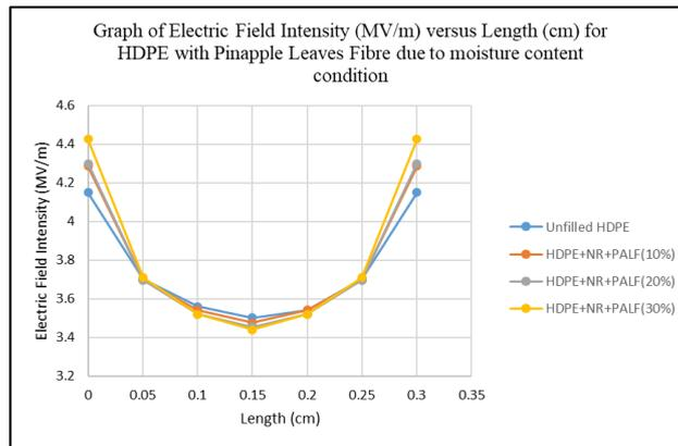
**Fig. 8 - Electric field intensity for HDPE with 10%, 20%, and 30% of pineapple leaves fibre with unfilled HDPE as a reference due to moisture content condition**
