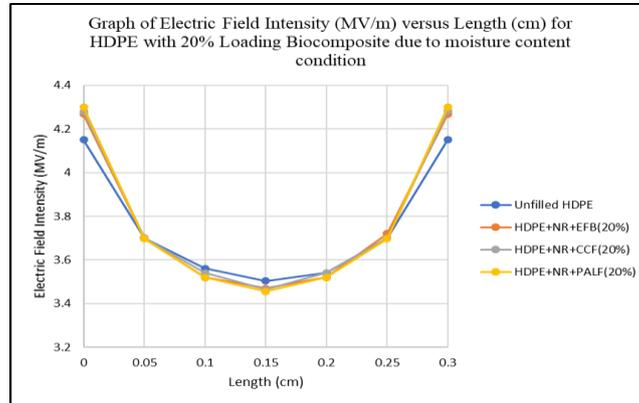
**Fig. 10 - Comparison of electric field intensity for sample HDPE with 20% loading of biocomposites due to moisture content condition**
