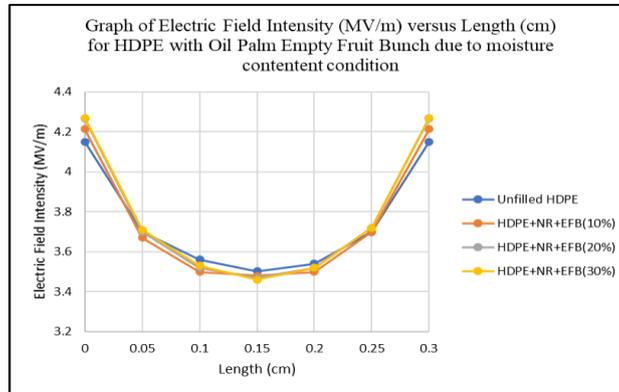
Fig 6 - Electric field intensity for HDPE with 10%, 20%, and 30% of oil palm empty fruit bunch with unfilled HDPE as a reference due to moisture content condition
