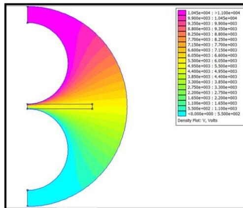
**Fig. 5 - Color density plot of voltage rendered in the electrostatic post-processor**
