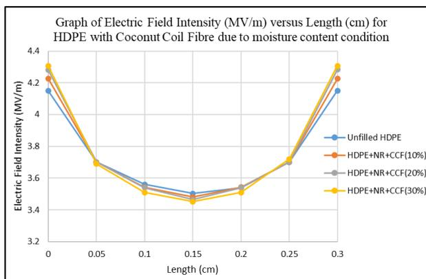
Fig. 7 - Electric field intensity for HDPE with 10%, 20%, and 30% of coconut coir fibre with unfilled HDPE as a reference due to moisture content condition
