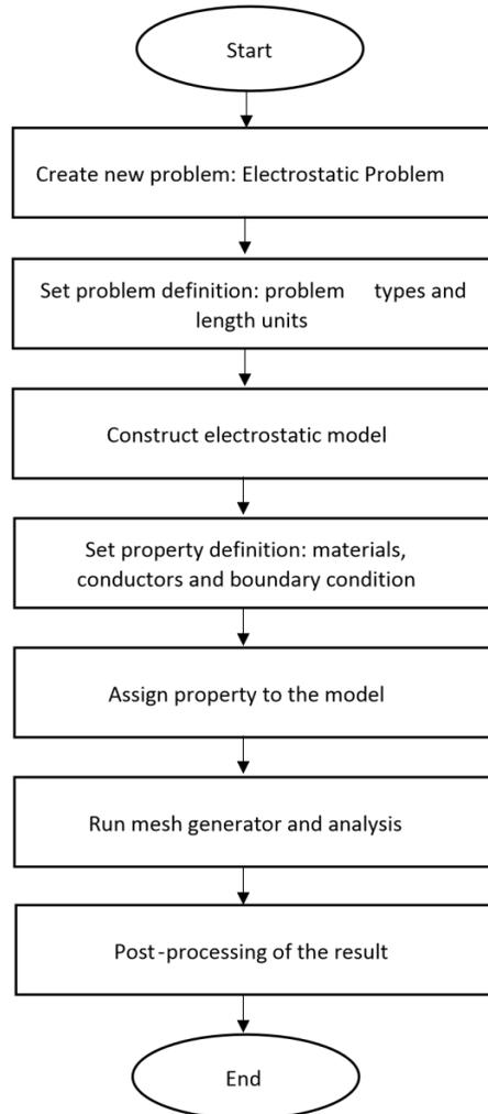
**Fig. 3 - Step for designing 2D axisymmetric problems in electrostatics**
