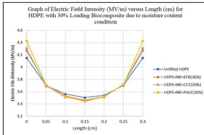
**Fig. 11 - Comparison of electric field intensity for sample HDPE with 30% loading of biocomposites due to moisture content condition**
