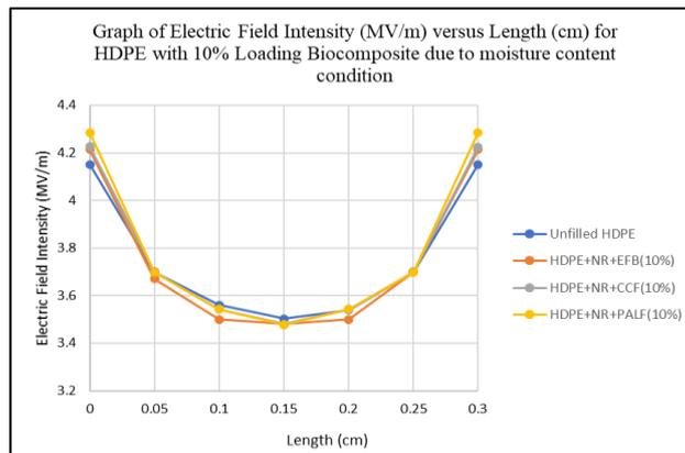
**Fig. 9 - Comparison of electric field intensity for sample HDPE with 10% loading of biocomposites due to moisture content condition**
