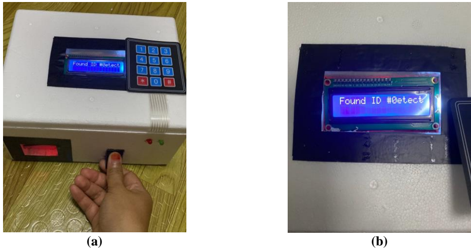
Fig. 3 - Fingerprint scanner as the second level security system (a) fingerprint scanning; (b) fingerprint is matched
