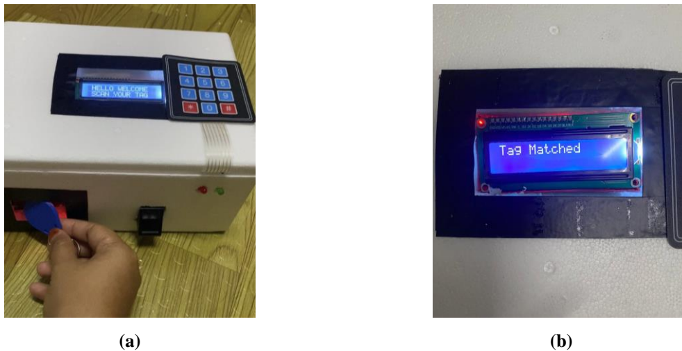
Fig. 2 - RFID module as the first level security system (a) scanning the RFID tag; (b) RFID tag is matched based on the LCD display
