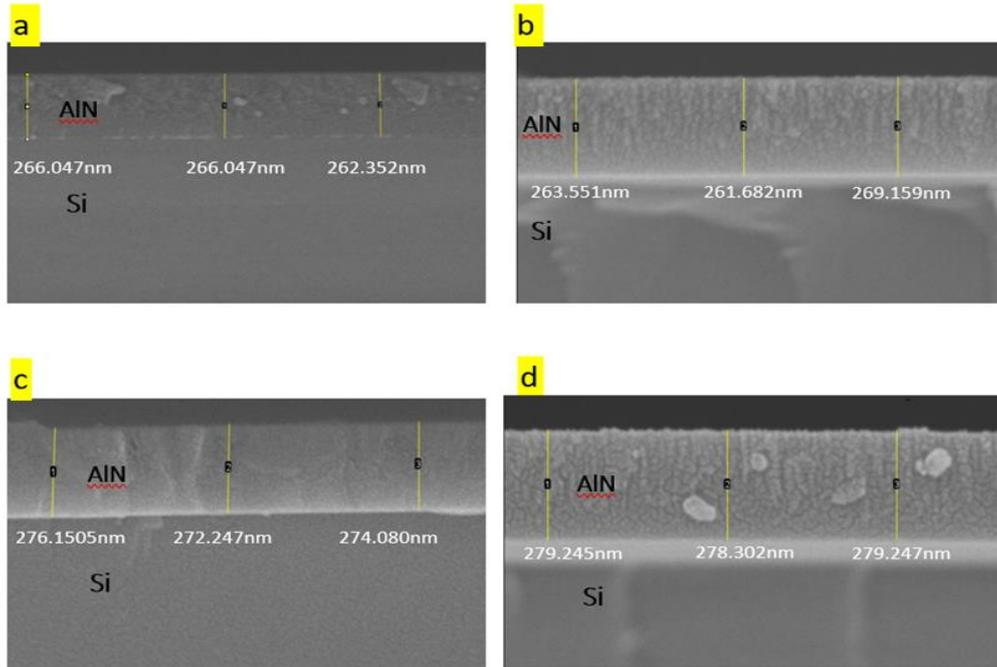
Fig. 7 - Cross-section by using FE-SEM in parameter 1
