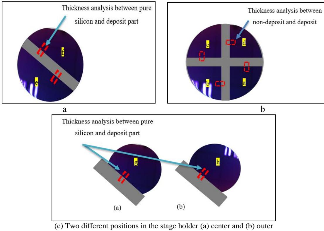
Fig. 5 - AlN film deposited by using RF magnetron sputtering with (a) parameter 1; (b) parameter 2 and; (c) parameter 3
