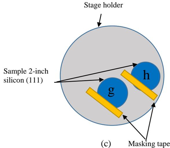
**Fig. 1 - The position of the sample on the stage holder (a) parameter 1, (b) parameter 2 and (c) parameter 3**
