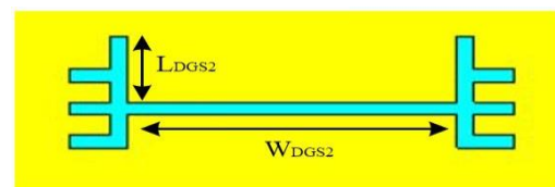
Fig. 5 - A single slot DGS connecting a pair of inverted U-shaped and inverted F-shaped DGS
