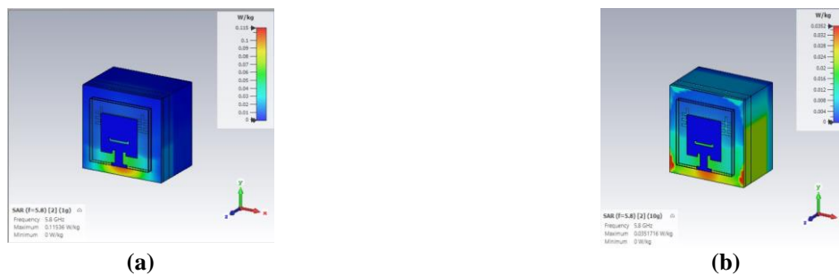
Fig. 19 - Simulated SAR values for the miniaturized dual-band dual mode microstrip patch antenna with DGS at 5.8 GHz for: (a) 1g of human tissue; (b) 10 g of human tissue
