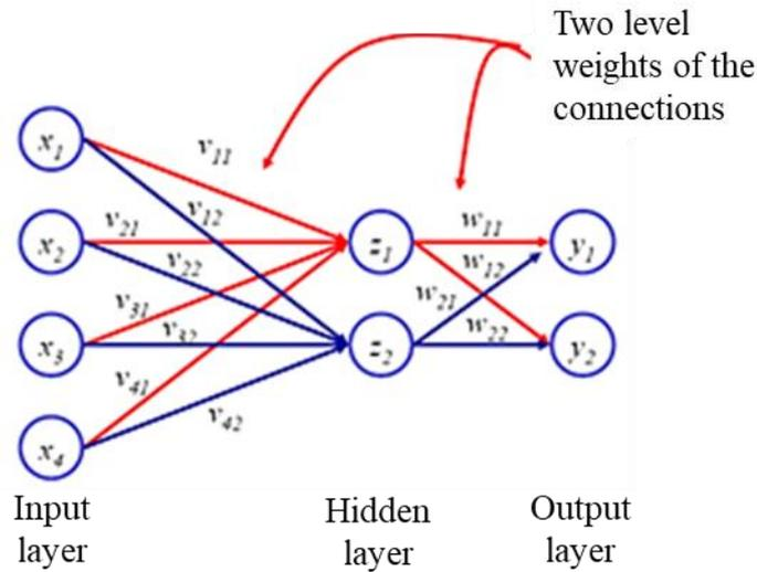
**Fig. 3 - Multi-layer neural network architecture.**
