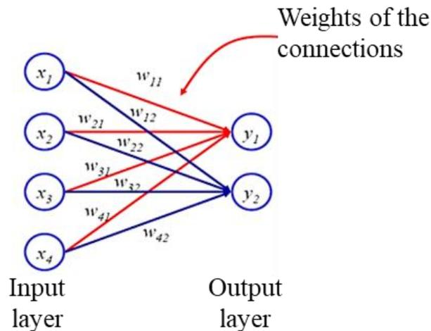
**Fig. 2 - One-level neural network architecture.**
