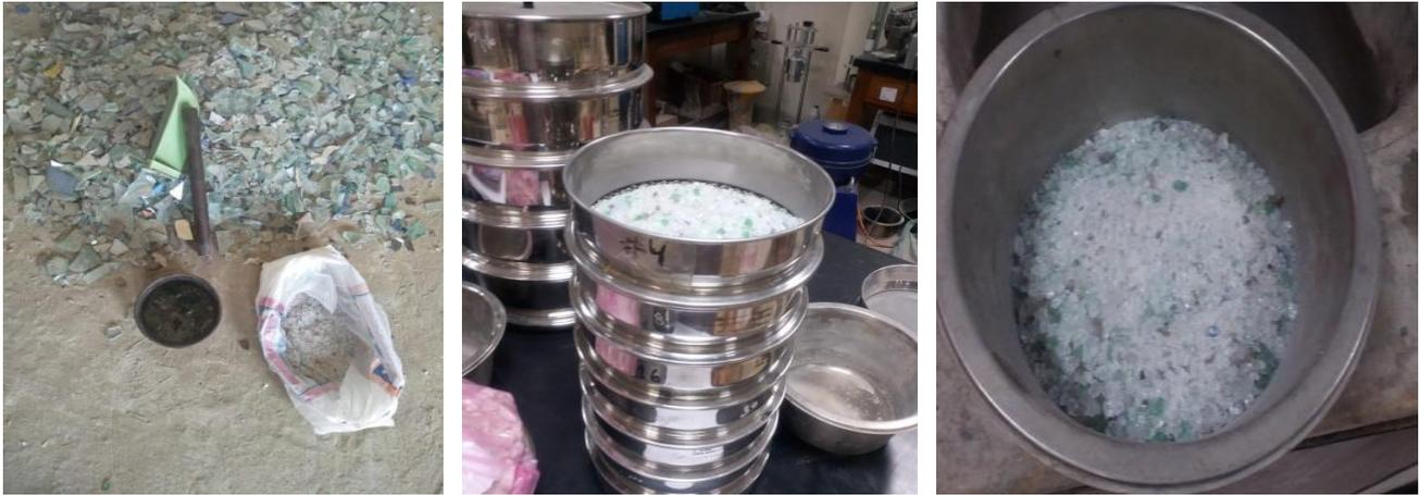
**Fig. 1 - Preparation of Recycled Waste Glass (RWG)**
