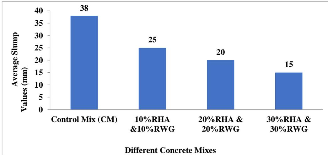
Fig. 3 - Average slump values of different concrete mixes
