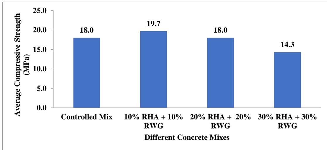
**Fig. 4 - Average compressive strength of cubical specimen at 28 days (MPa)**
