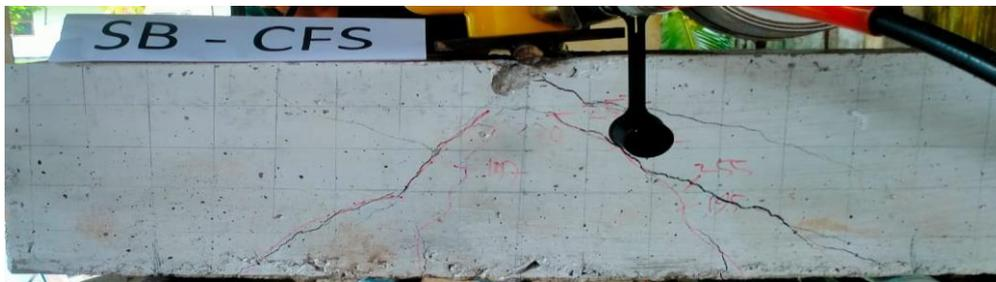
**Fig. 9 - SB-CFS crack pattern**
