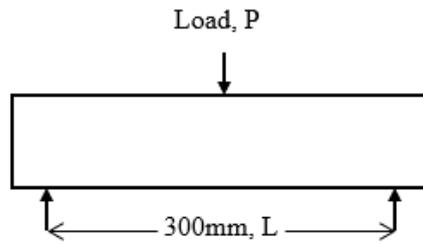
**Fig. 2 - Schematic drawing of three-point bending test**
