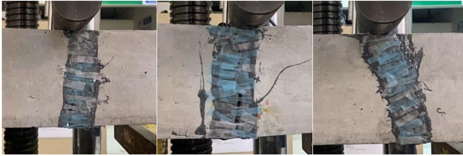
**Fig. 7 - Failure after repaired (2nd Method)**
