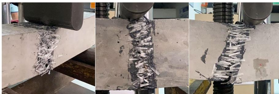
**Fig. 6 - Failure after repaired (1st Method)**
