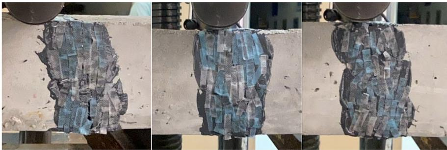
**Fig. 8 - Failure after repaired (3rd Method)**
