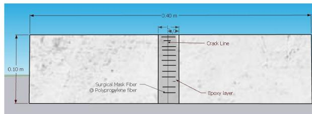
**Fig. 3 - Schematic drawing 1<sup>st</sup> and 2<sup>nd</sup> method**
