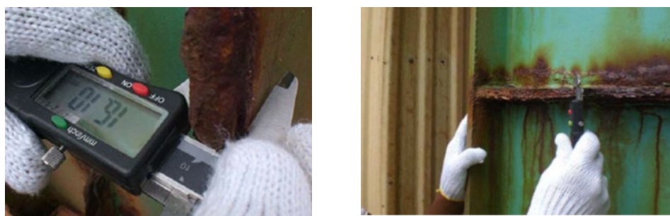
Fig. 4 Vernier calliper measurements
