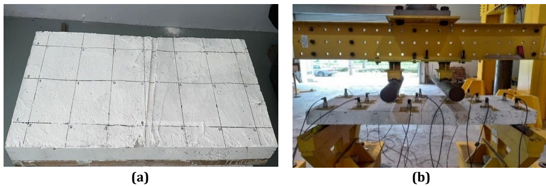
Fig. 2 Sample of slab (a) Gridlines on the slab; (b) Location of the accelerometer
