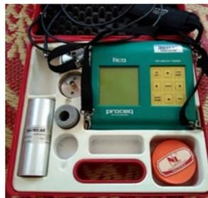
**Fig. 1** Schmidt rebound hHammer **Fig. 2:** proceq ultrasonic tester
