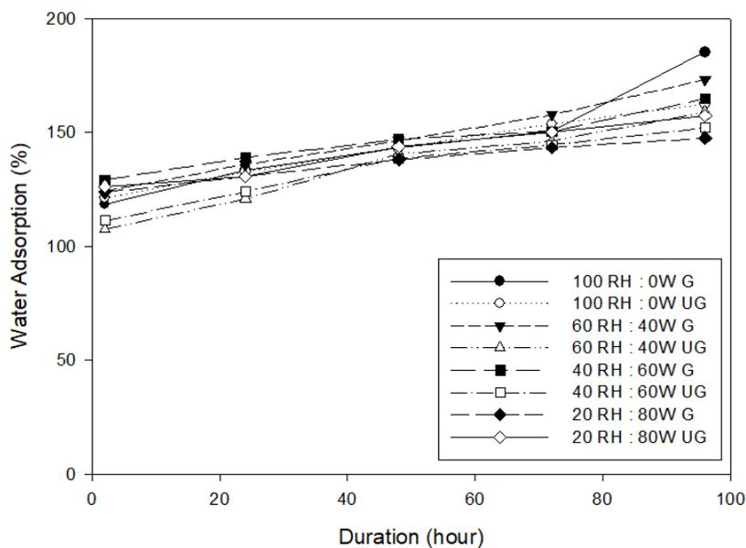
Fig. 2 - Water absorption of particleboard
