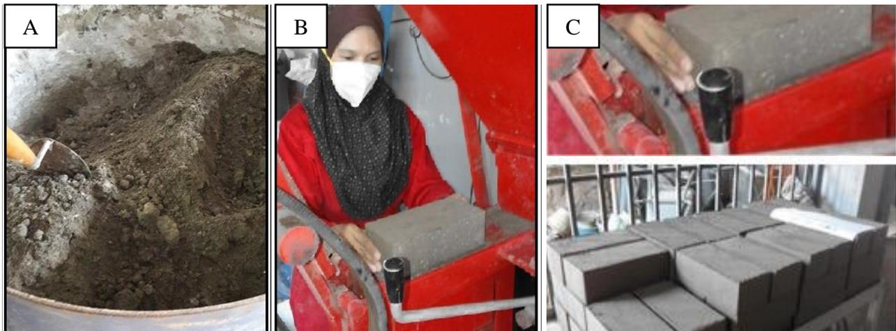
**Fig. 1 - Fabrication of unfired bricks (a) target materials, stabilizer, and water were mixed thoroughly in a mixer; (b) the mixture was pressed at 25 MPa and fresh brick was pressed out from mould; (c) fresh unfired bricks**
