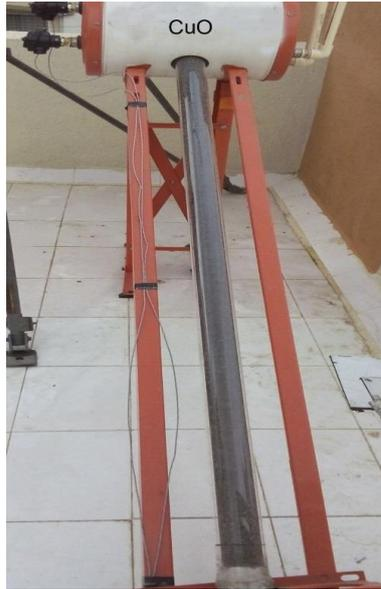
**Fig. 5 - CuO nanoparticles coated ETC experimental set up**
