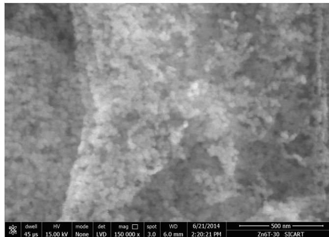
Fig. 2 - SEM micrograph of CuO nanoparticles
