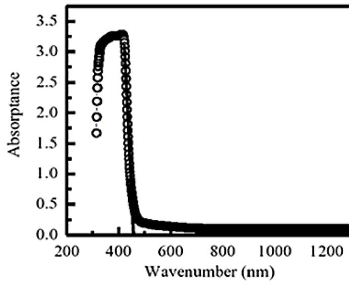
**Fig. 4 - UV-Vis absorption spectra of CuO nanoparticles synthesized on glass substrate**
