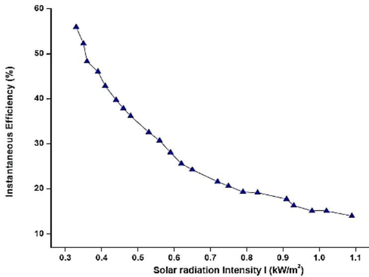
Fig. 9 – Performance curves of instantaneous efficiency vs solar radiation intensity (I)
