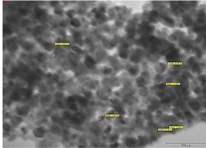
**Fig. 3 - TEM micrograph of CuO nanoparticles**
