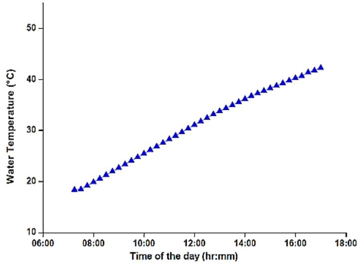
Fig. 7 – ETC instantaneous tube water temperature vs daytime
