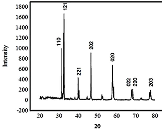
Fig. 1 - XRD pattern of CuO nanoparticles
