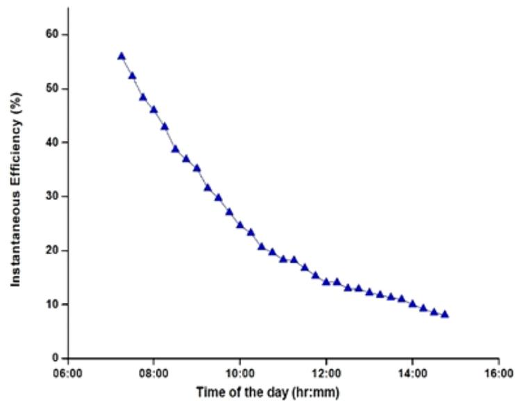
**Fig. 6 - CuO nanoparticles coated solar evacuated efficiency vs daytime**
