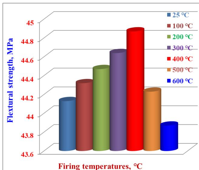
**Fig. 5** Flexural strength of the optimum cement pastes containing 20 % CSPW hydrated up to 90 days and subjected to different firing temperatures
