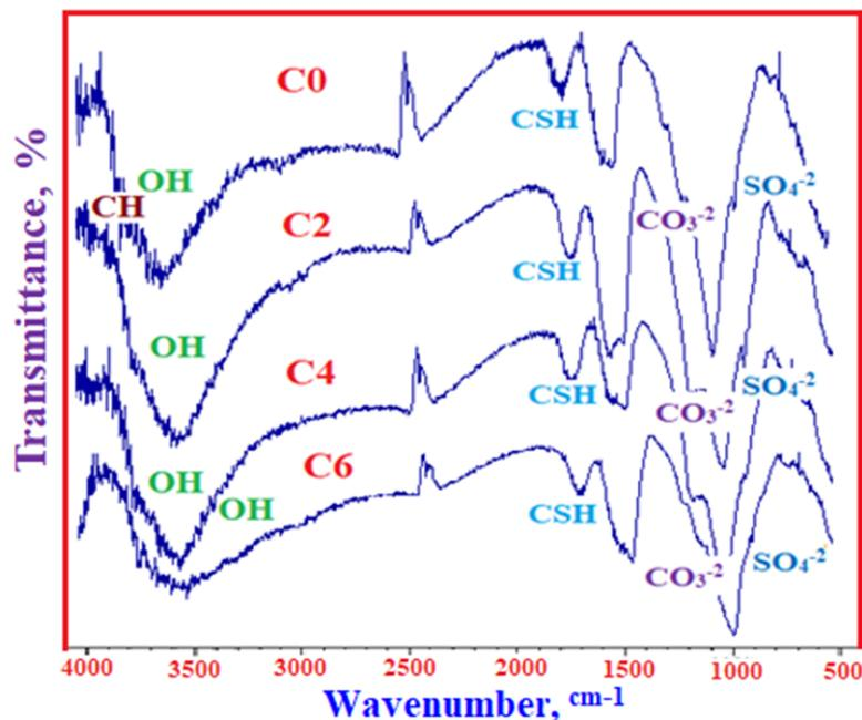
Fig. 7 FT-IR spectra of the cement pastes C0, C2, C4 and C6 fired up to 25, 200, 400 and 600 °C
