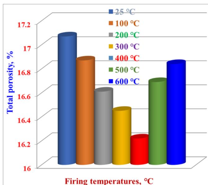
**Fig. 3** Total porosity of the optimum cement pastes containing 20 % CSPW hydrated up to 90 days and subjected to different firing temperatures
