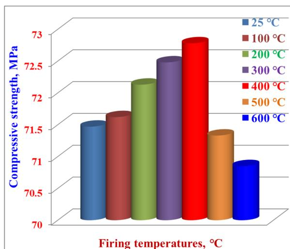
**Fig. 6** Compressive strength of the optimum cement pastes containing 20 % CSPW hydrated up to 90 days and subjected to different firing temperatures
