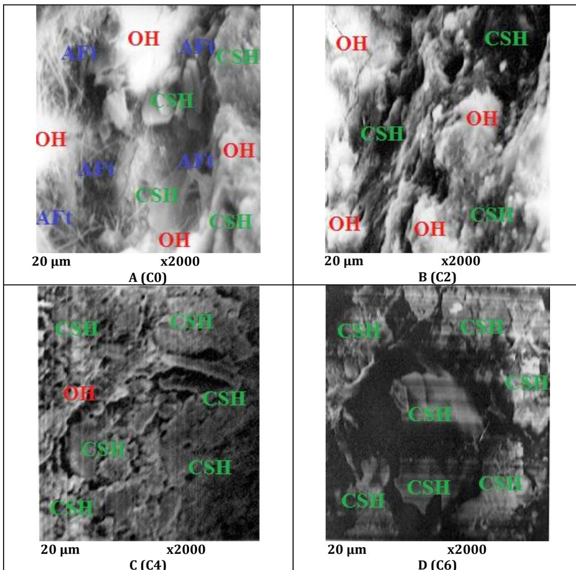
**Fig. 8** SEM images of C0, C2, C4 and C6 cement pastes with and without CSPW after the exposure to firing temperatures
