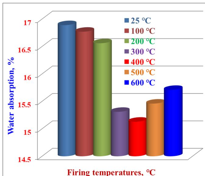
**Fig. 2** Water absorption of the optimum cement pastes containing 20 % CSPW hydrated up to 90 days and subjected to different firing temperatures
