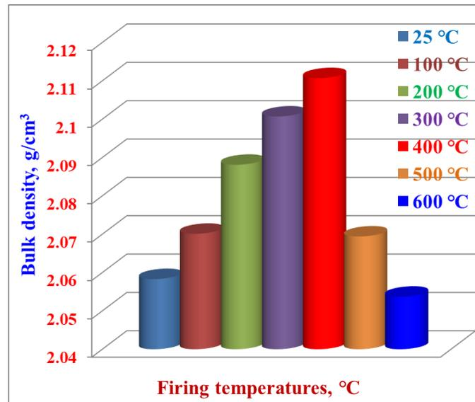
**Fig. 4** Bulk density of the optimum cement pastes containing 20 % CSPW hydrated up to 90 days and subjected to different firing temperatures
