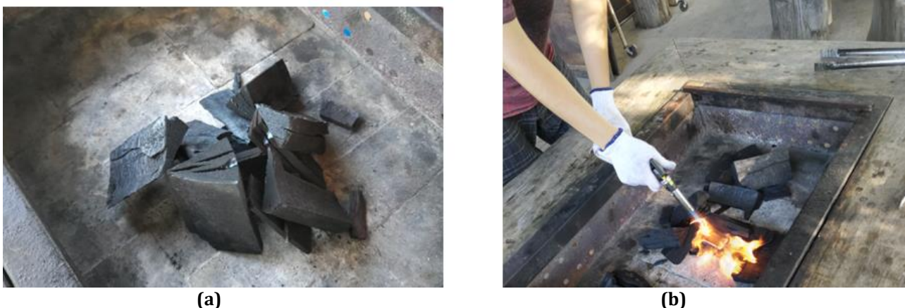
Fig. 3 (a) Arranged charcoal before ignition; (b) Fire ignition with LPG gas cylinder
