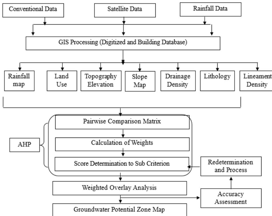
Fig. 3 Flowchart showing the methodology adopted for the use of remote sensing in groundwater exploration [31]
