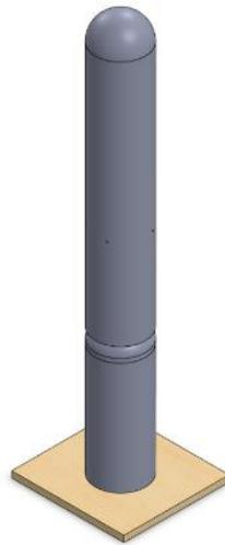
Fig. 2 - Isometric view of vortex bladeless wind turbine
