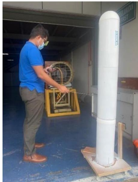
Fig. 4 - Testing of VBWT on Different Windspeed
