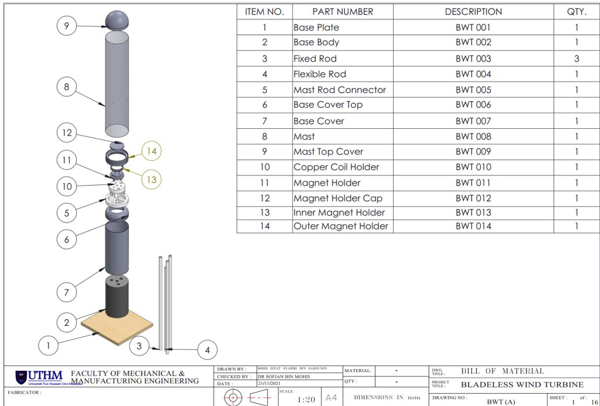
Fig. 5 - (a) Exploded view of final VBWT design
