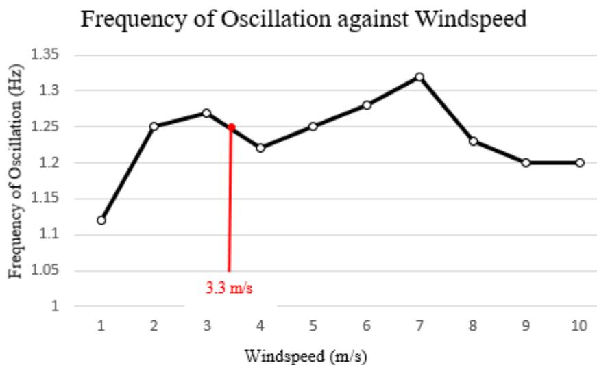
**Fig. 8 - Intersection of resonance windspeed and oscillation frequency**
