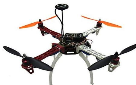
**Fig. 1** The F450 quadrotor used for this project with the Pixhawk-based autopilot system
