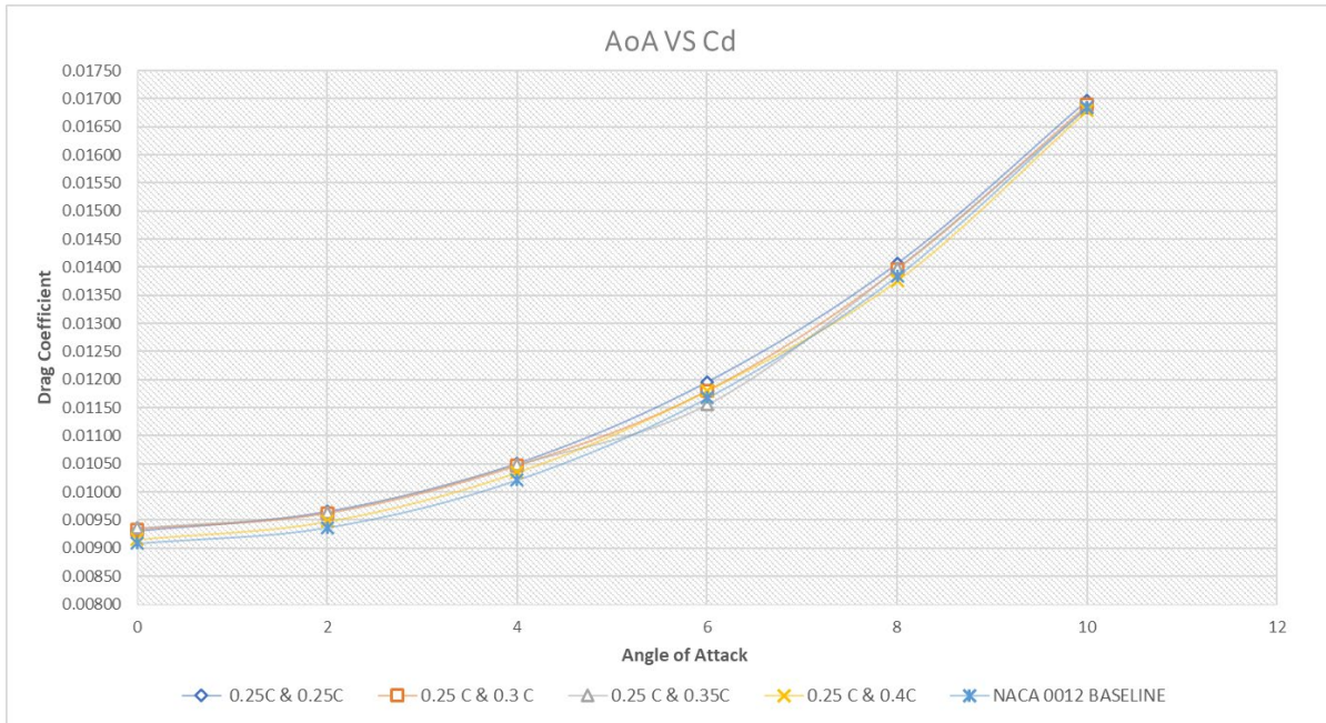
Fig. 19 Drag coefficient ( Cd ) vs. angle of attack (AOA) for different parallel groove positions (0.25C) and NACA 0012 baseline
