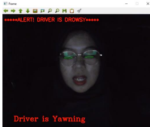
Figure 10: Drowsiness detection of a spectacled driver at night
