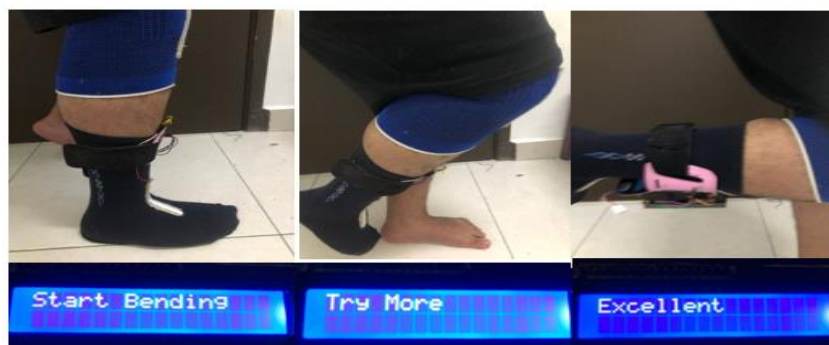
Figure 14: LCD displays the status of knee bending
