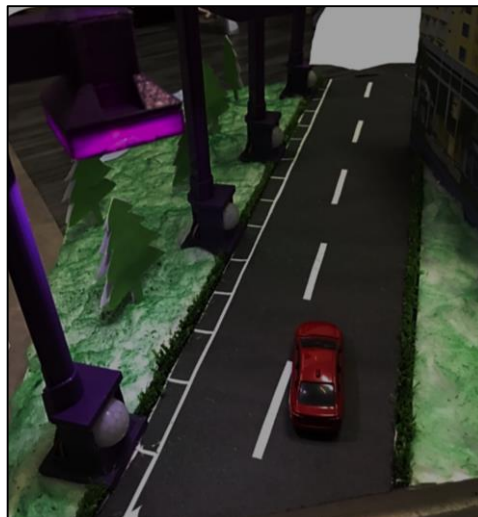
Figure 2: Streetlight is turned on when motion detected
