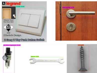
Figure 9: The Result of Run Inference with Yolov3-Tiny Trained Weights
