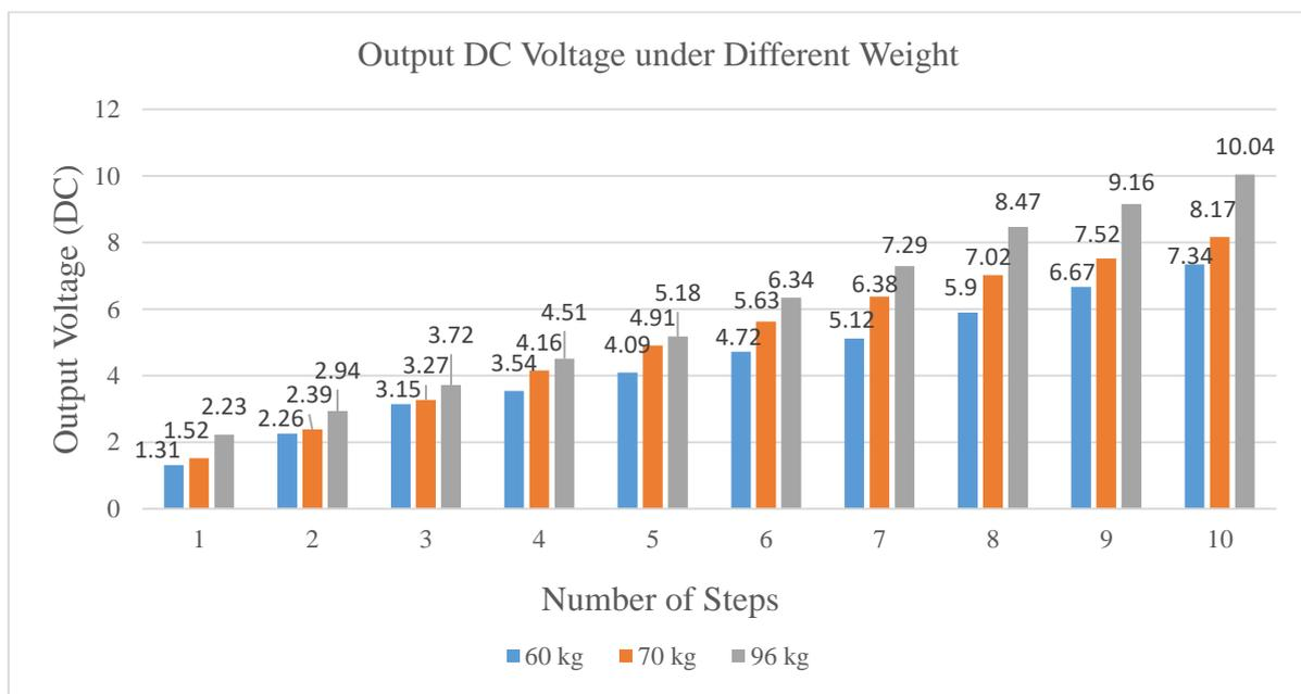
**Figure 12: Graph of output DC voltage under three different weights**
