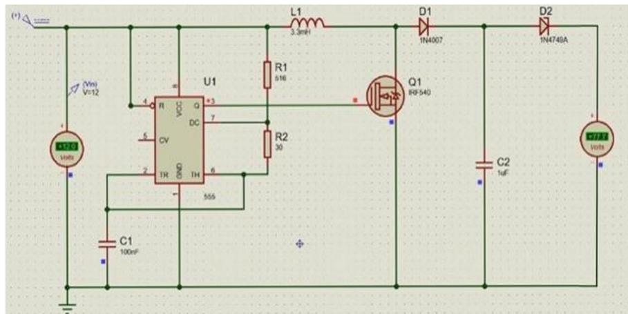
**Figure 8: Schematic circuit of dc-dc boost converter**
