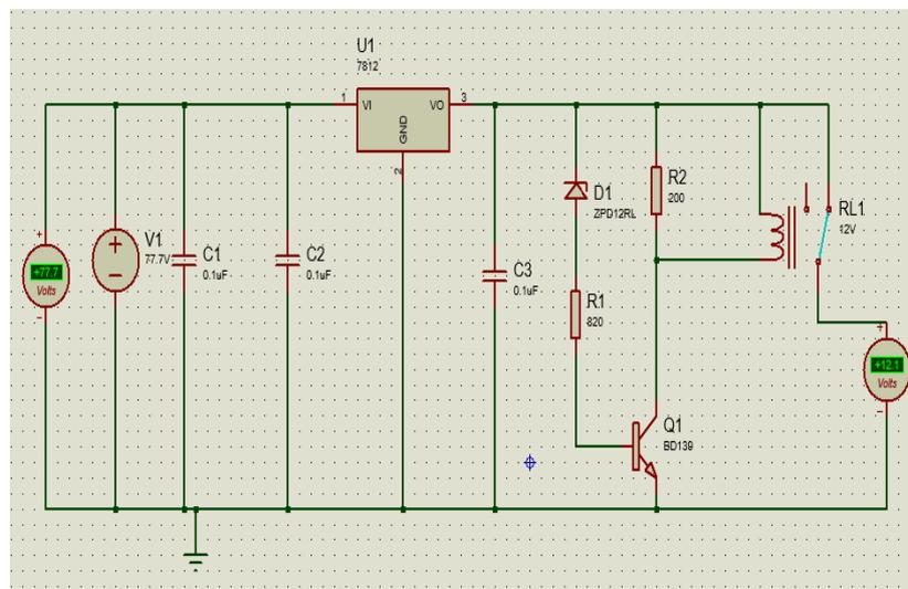
**Figure 9: Schematic circuit of voltage regulator and charging circuit**
