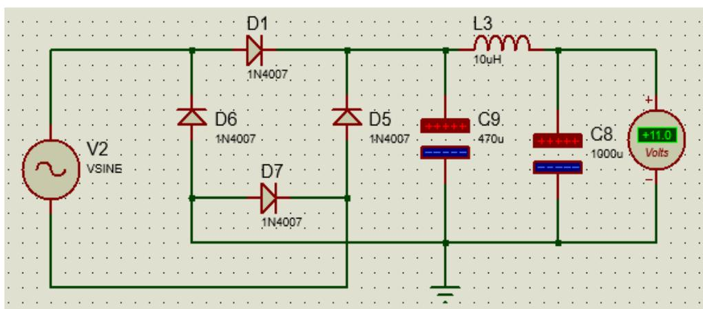
Figure 5: Schematic circuit of ac-dc converter with pi-filter circuit
