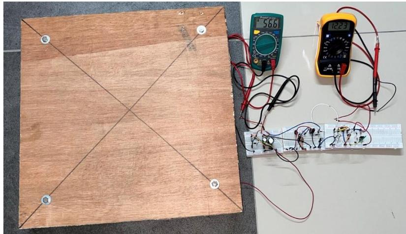
**Figure 15: Prototype arrangement of the energy harvesting system**
