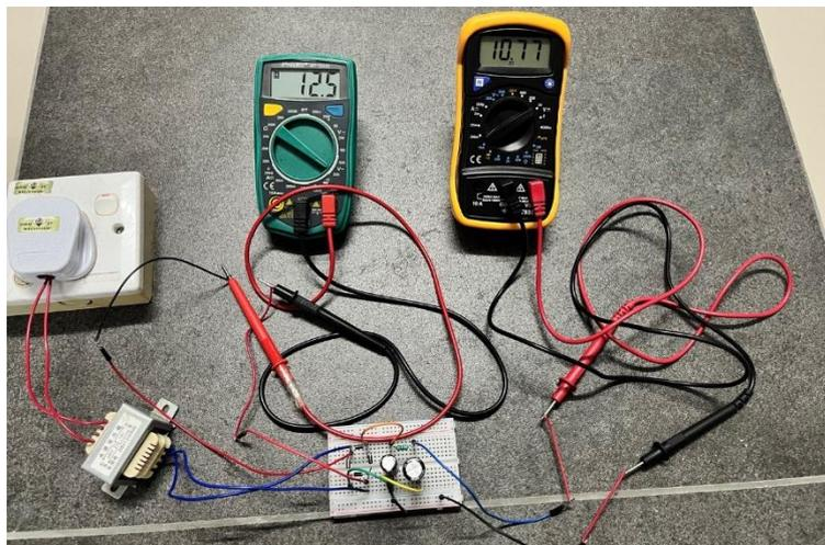
**Figure 11: Performance of full-wave bridge rectifier with pi-filter circuit**
