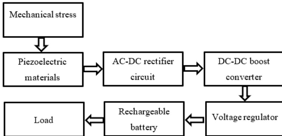
**Figure 1: Block diagram of the proposed system for piezoelectric energy harvesting system**
