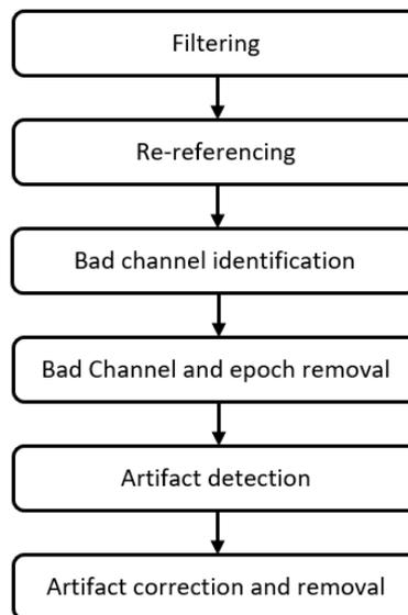
**Figure 1: EEG preprocessing pipeline**
