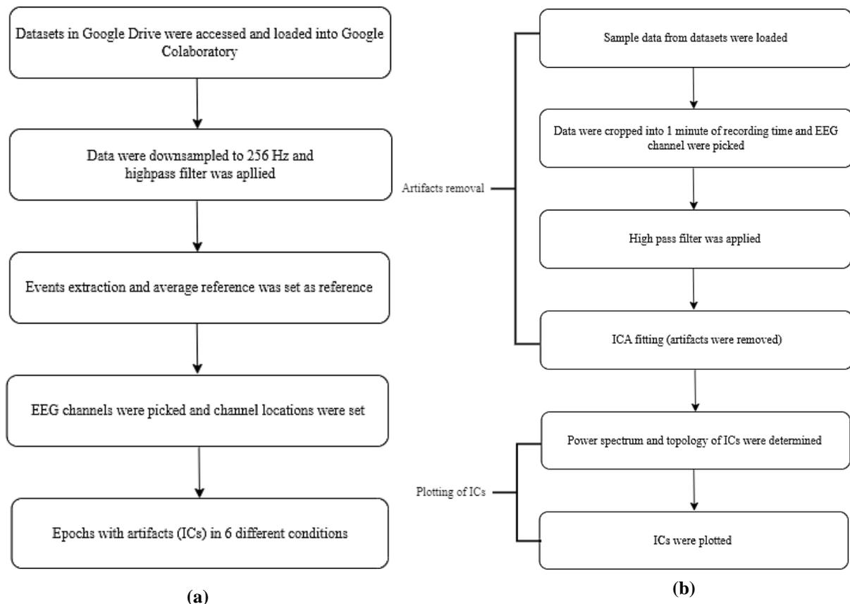
**Figure 2: Simulation process (a) First coding; (b) Second coding**
