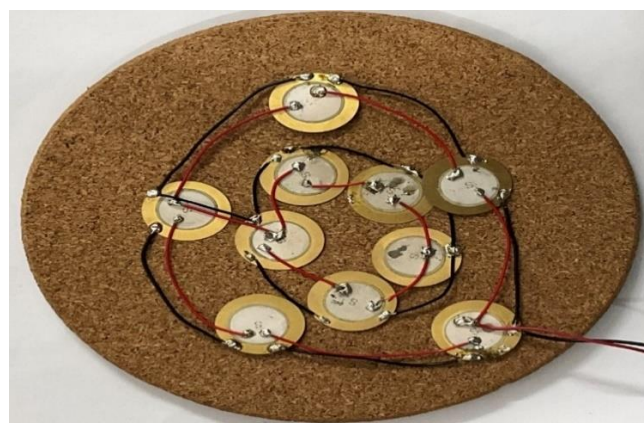
Figure 2: Final prototype of the piezoelectric generator
