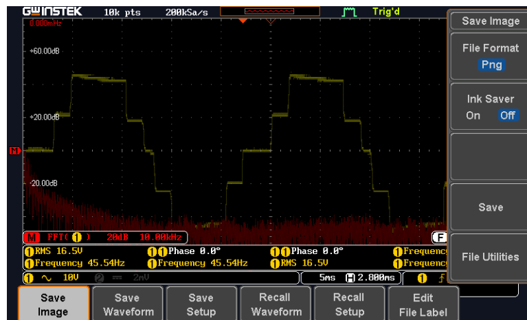
Figure 8: Hardware Output Voltage of 5-Level Multilevel Inverter
