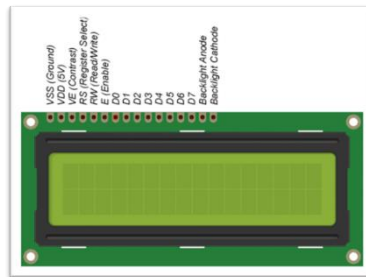
Figure 3: 16x2 LCD display pin configuration.
