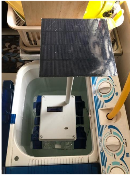
Figure 9: Floating backup supply using solar.
