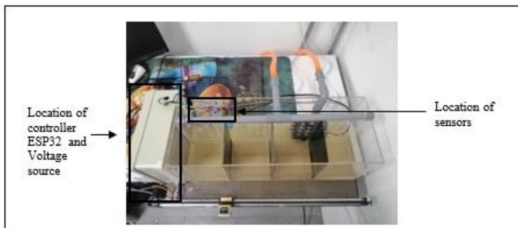
Figure 8: System controller of this project
