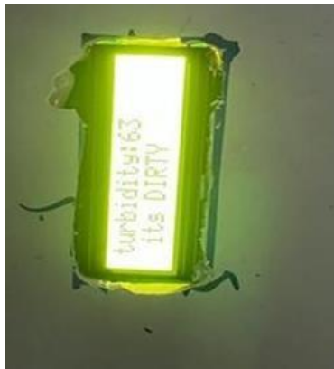
Figure 7: Monitor Showing Reading of Turbidity
