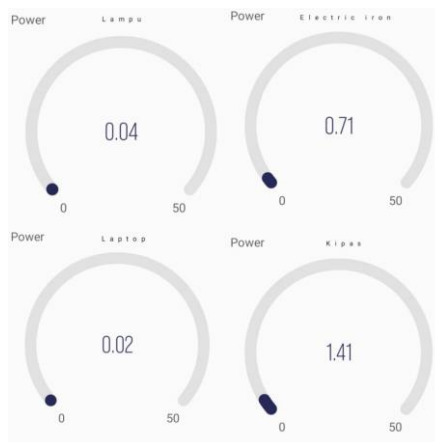
Figure 8: Power reading taken using prototype device for each load
