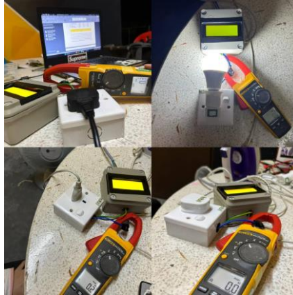
Figure 5: Current reading was taken using Fluke 375 Clamp Meter for each load
