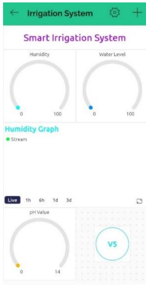
Figure 4: User interface design of the monitoring system in the Blynk application.
