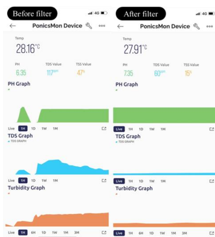
Figure 13: Water quality Blynk monitoring before and after filtration
