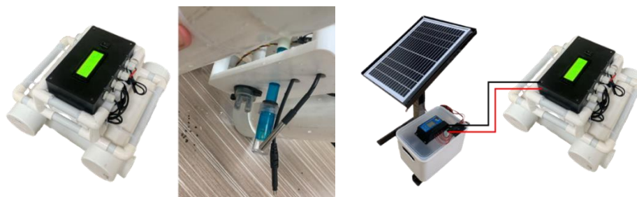
Figure 12: Solar charge PonicsMon device prototype
