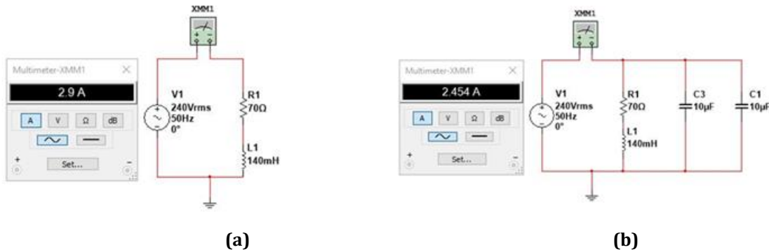
Fig. 8 Current of hair dryer circuit (a) before adding capacitor; (b) after adding capacitor
