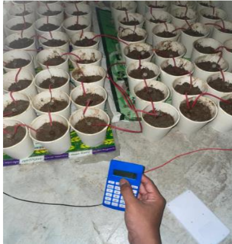
Figure 11: Calculator turn on after connected by soil as voltage source without using any conventional battery
