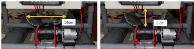
Figure 7: The dimension of the conveyor
