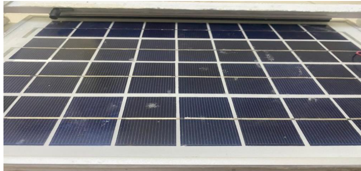
Figure 10: Surface solar photovoltaic panel after cleaning
