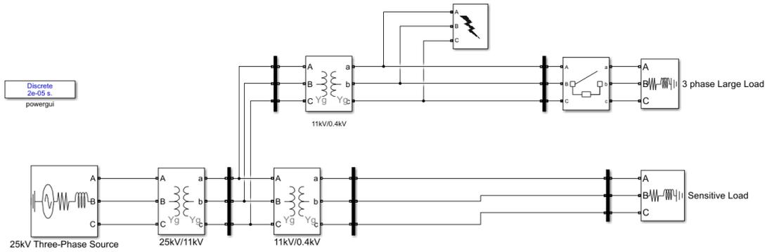
**Figure 2: Modified test case with TPF**
