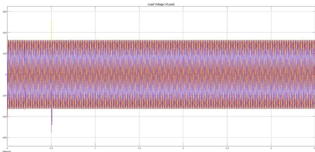
**Figure 10: Sensitive load voltage during mitigation process of TPF**
