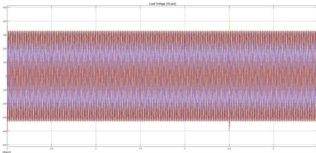
**Figure 12: Sensitive load voltage waveform during the mitigation process of switching on heavy load**
