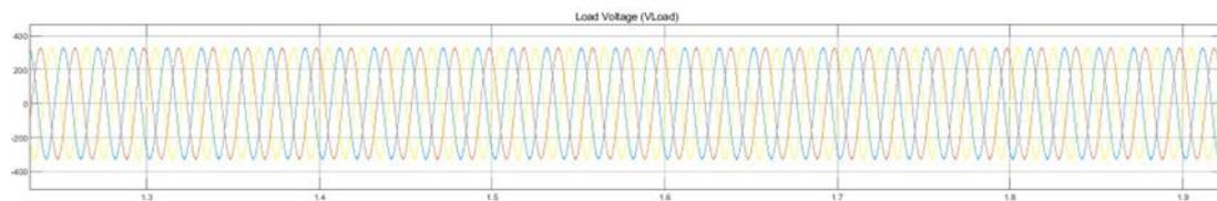
Figure 7: Sensitive load voltage waveform under normal condition
