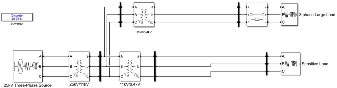
**Figure 3: Modified test case with switching on heavy load**
