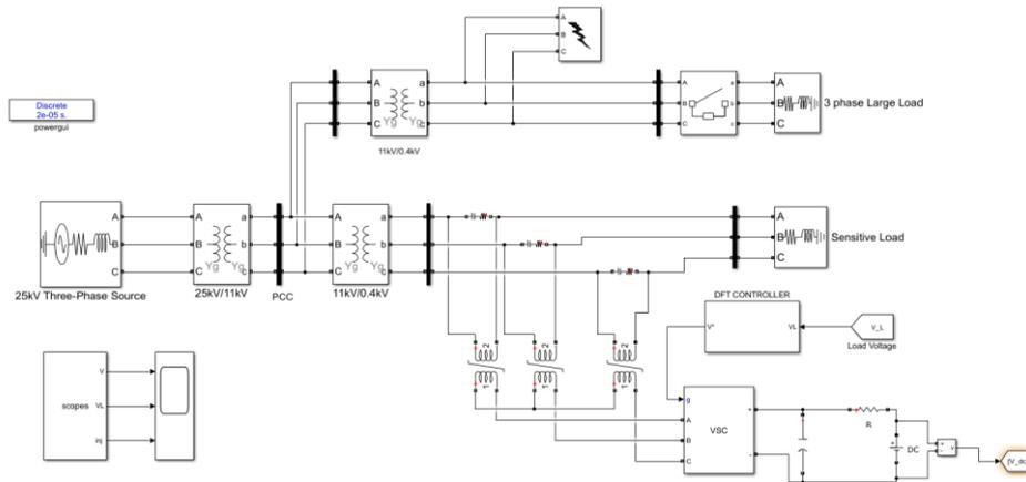
**Figure 4: Modified test case with DVR connected**
