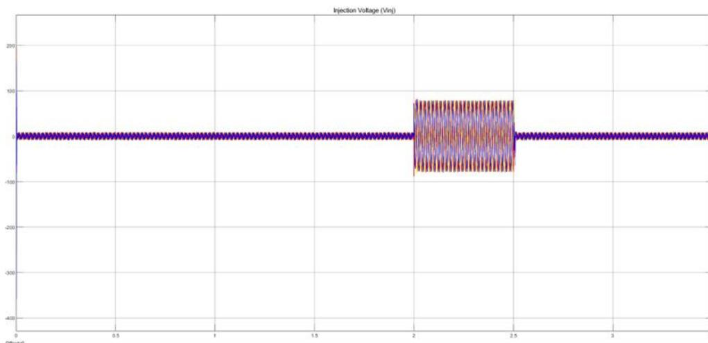
**Figure 13: Injection voltage from DVR during the mitigation process of switching on heavy load**
