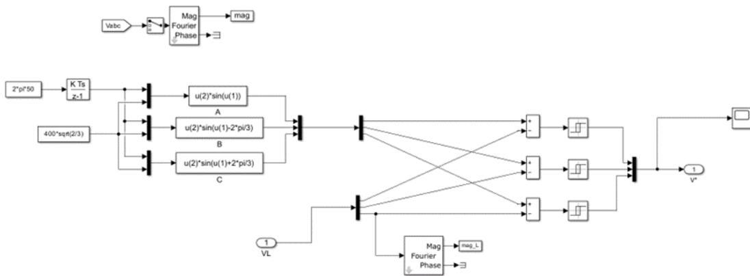
Figure 6: Model of DFT algorithm control circuit
