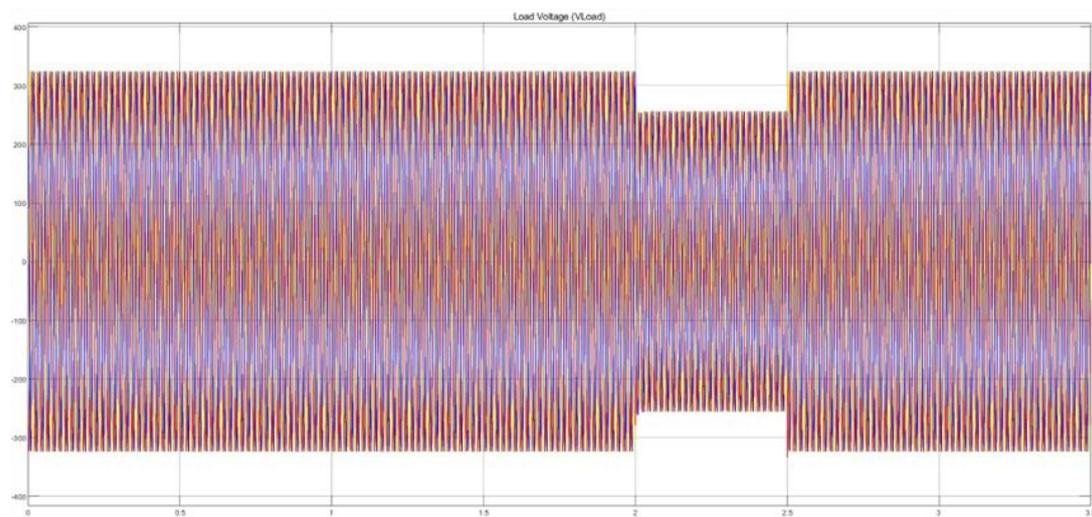
**Figure 9: Sensitive load voltage during the switching on heavy load**
