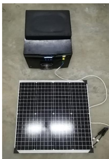
Figure 11: Physical setup to test the solar charging system.
