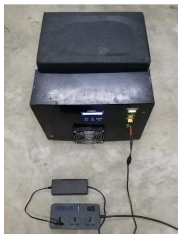
Figure 9: The setup to perform the charging process by using an adaptor.
